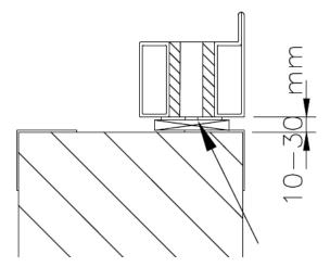
The frame is prepared with mounting holes ø15 mm and underlying mounting brackets ø8.5 mm, where the frame is to be attached. Drill holes (ø10 mm for concrete, lightweight concrete, block wall or masonry or ø6.5 mm for steel skeleton wall) in the masonry through the mounting holes and secure with the supplied fasteners.
