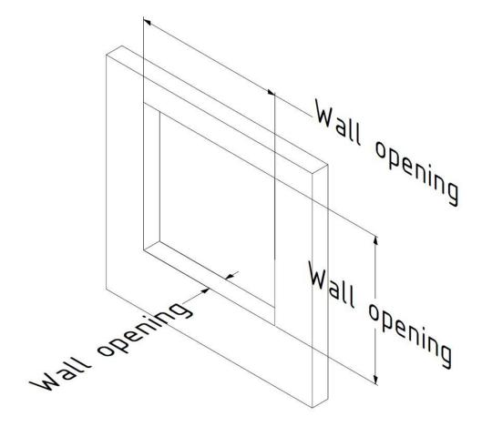
The sealing width is the distance between the window frame and the wall. The distance must not be less than 10 mm or more than 30 mm in any place – see the figure below.
