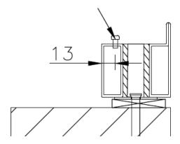
Put window sealing on profiles and glass strips. The window must have 2 layers of 4 mm window sealing on the glass strip and 1 layer of 4 mm window sealing on the frame.
