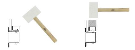
A sloping base profile can be mounted over the horizontal glass strip. The sloping bottom profile is pressed down between the glass and the glass strip. The window seal must be mounted on the sloping bottom profile towards the glass before it is pressed down between the glass and the glass strip.
