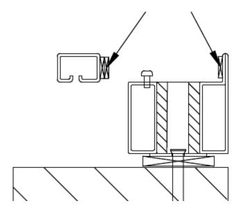
If there is a problem with space, use window sealing with a thickness of 1, 2, 3 or 4 mm.
