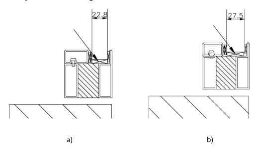
After mounting the glass block and glass, the glass strip must be applied to hold the glass in place in the frame. The glass strip is assembled with 90° joint in corners and at any bars. Horizontal glass strip should be full-length.
