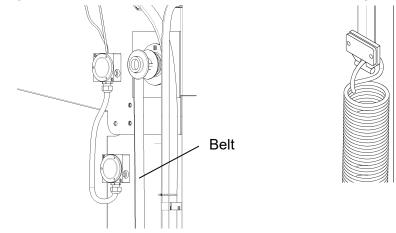
At wide doors a spring along the frameleg opposite the motor side is also mounted. Before mounting the spring the curtain should be in the top, the door is now fully open. The spring is mounted the same way as the spring in the motorside (see above).
