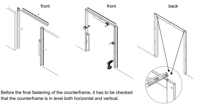
The counter frame is prepared with mounting holes and underlying mounting connectors where the counterframe has to be fastened. Drill holes through the mounting holes and fasten the counterframe with the supplied fasteners.
