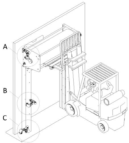
Make sure the frame legs are in level before fastening them to the wall and floor. The frame legs are fastened the the prepared holes with the delivered fasteners.
