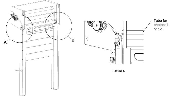
The top frame is placed between the frame legs beneath the roll. The heating cables are pulled through the frame leg and into the connectorbox on the frame leg. The top frame is fastened to the frame legs with the delivered angle brackets and to the wall with the delivered fasteners.
