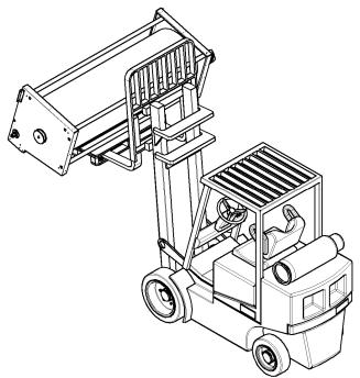
The roll is liftet up against the wall above the wall opening. The frame legs are fastened to the roll with the delivered M10 bolts -4 in each side.
