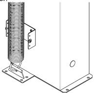
The top of the spring is mounted to a connector on the belt (the belt is fastened on the axel of the roll). By adjusting the placement of the connector on the belt the spring is prestressed 50 mm.
