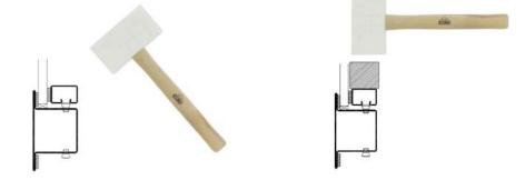
A sloping base profile can be mounted over the horizontal glass strip. The sloping bottom profile is pressed down between the glass and the glass strip. The window seal must be mounted on the sloping bottom profile towards the glass before it is pressed down between the glass and the glass strip.
