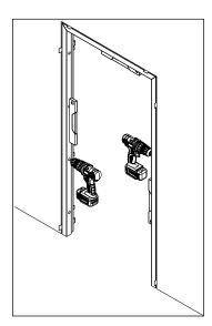
Fasten the frame through the existing mounting holes and underlying mounting connectors in the frame. Drill holes through the mounting holes and fasten the frame with the supplied fasteners. Any counter frame is also fastened through the prepared holes for mounting.
