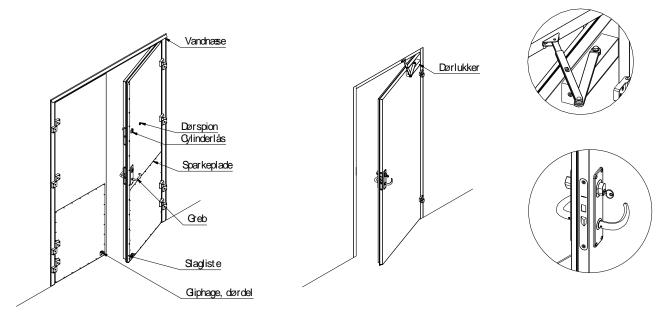
When the frame is mounted in the wall opening and all measurements are checked, the door leaf is mounted on the hinges on the frame. The hinges are lubricated with grease (optionally Food Grease).
