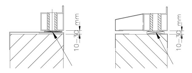
The frame is prepared with mounting holes ø15 mm and underlying mounting brackets ø8.5 mm, where the frame is to be attached. Drill holes (ø10 mm for concrete, lightweight concrete, block wall or masonry or ø6.5 mm for steel skeleton wall) in the masonry through the mounting holes and secure with the supplied fasteners. The frame MUST be fixed in a fire wall.
