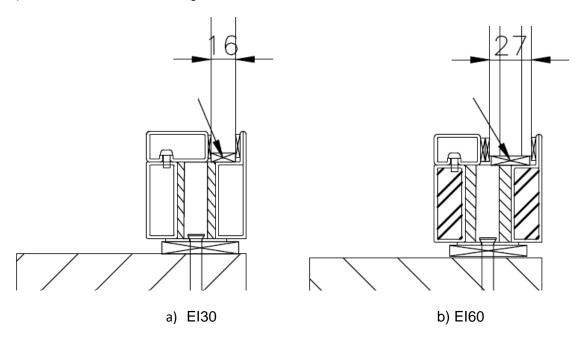
After mounting the glass block and glass, the glass strip must be applied to hold the glass in place in the frame. The glass strip is assembled with 90° joint in corners and at any bars. Horizontal glass strip should be full-length.
