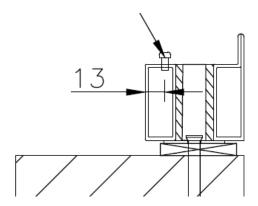
Put window sealing on profiles and glass strips.
