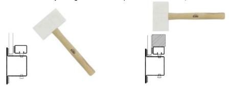
A sloping base profile can be mounted over the horizontal glass strip. The sloping bottom profile is pressed down between the glass and the glass strip. The window seal must be mounted on the sloping bottom profile towards the glass before it is pressed down between the glass and the glass strip.
