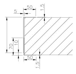
U – flashing in 2 parts (if wall thickness is varied).
