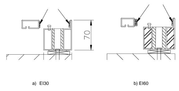
If there is a problem with space, use window sealing with a thickness of 1, 2, 3 or 4 mm.
