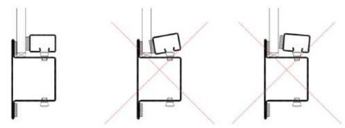
Hit one end of the glass strip. Hit the edge of the glass strip and directly over the glass strip screw. If the glass strip is hard to hit, try using a wooden or plastic block to help.
